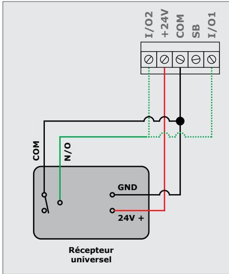
IMAGE 84. CÂBLAGE D'UN RÉCEPTEUR UNIVERSEL SUR LE SDO4 SMART
