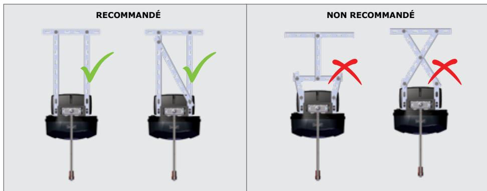
IMAGE 34. CONFIGURATIONS DE MONTAGE CORRECTES ET INCORRECTES
