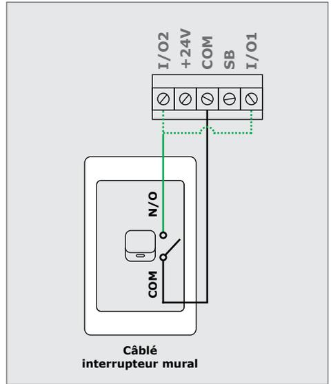
IMAGE 85. CÂBLAGE D'UN INTERRUPTEUR MURAL AU SDO4 SMART
