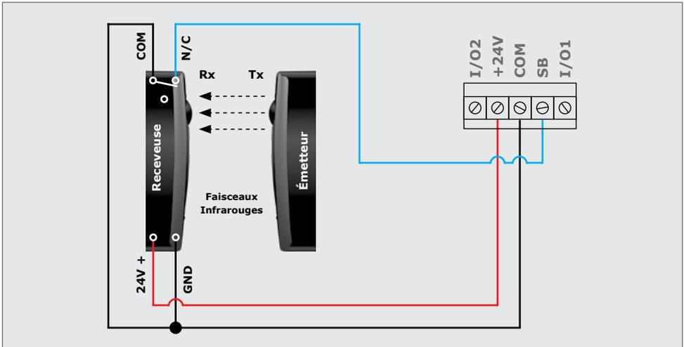
IMAGE 82. CÂBLAGE DES CELLULES DE SÉCURITÉ PHOTON SUR LE SDO4 SMART (QUATRE FILS)
