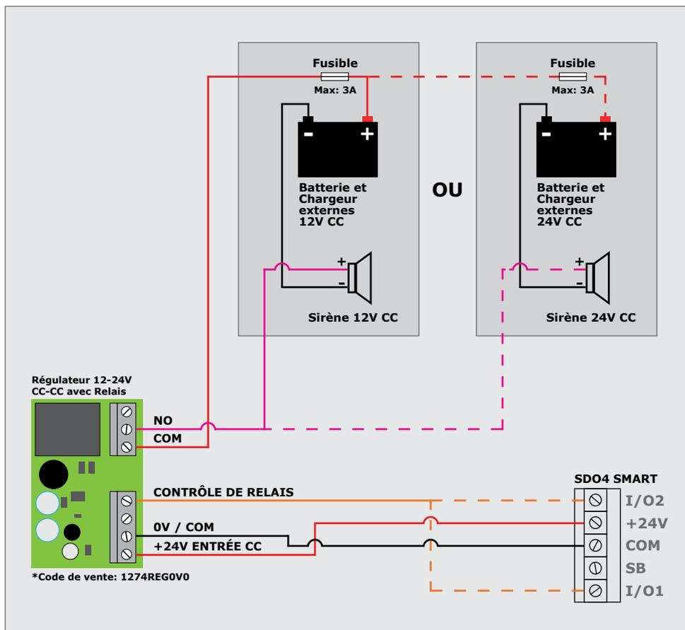
IMAGE 87. CÂBLAGE ALARME ANTI-TAMPER AVEC SIRÈNE
